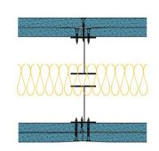
90/90 Minutes (Integrity/Insulation). BTC 17440F - BRE Report P102396-1011A Refer to Speedline Specification Clause 200 mm. (At Base Track, Excluding Finishes) Severe - Annexes A-F 67 RwdB, -10CtrDate Tested or Assessed Against - TWI50-B-60(50)(200)
